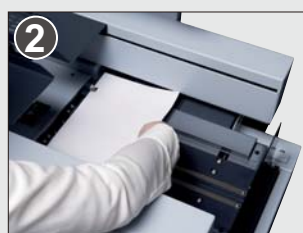
Place the cover and press the start button again.
