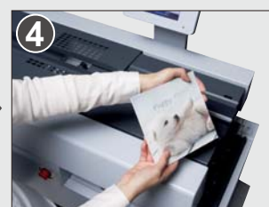
A cover is applied and book binding is completed.
