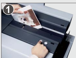
Insert the book block and press the start button.
