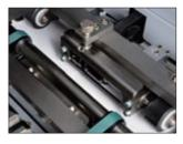
Scoring positions are automatically set to the input thickness. Scoring depth is easily adjusted to accommodate a wide range of cover stocks and thickness. This insures a professional bind quality with sharp, square spine corners.
