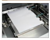
Top and bottom transport belts provide stable transportation of various cover types, and high-precision jog mechanisms register the cover securely for consistent, accurate binding. Strong and beautiful quality book... The quality is equivalent with commercial size binding system.
