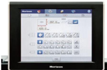
The 12.1 inch color touch-screen is icon-based for user-friendly operation. Set-up and operation can be done at the touchscreen. Up to 999 job settings can be stored in job memory. The job settings saved in the existing AFC-566F can be transferred to the AFV-566FKT/564FKT.
