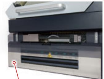
Covers on both sides of knife fold section can be opened.
