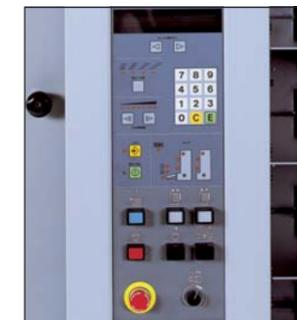
Horizon's highly advanced sensor and electronic controls make for adjustment-free, easy operation. Presetting of the number of completed sets per grouping, the total count, as well as placement of the front and back covers allows for flexibility or programming. State-of-the-art sensors detect such errors as miss or double sheet feeding, incorrectly aligned sheets, as well as imperfect sheets.
