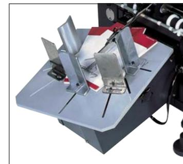
This tray automatically swings 30 degrees after delivery of each collated sequence, making it the perfect tray for jobs such as multi-page booklets. The receiving guides may be adjusted according to the scales provided, allowing for exact receipt of the collated sets. The tray descends automatically as its delivered pile increases. Maximum paper size for this tray is 470 mm x 318 mm (18.5" x 12.5").
