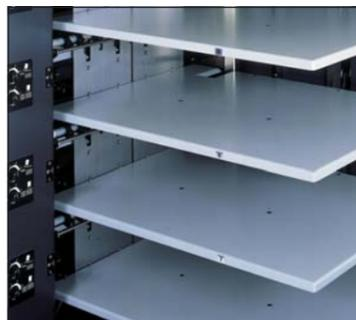
The high capacity feed stations provide maximum production in between re-loads. Accurate feeding is maintained by the easy accessible paper feed controls. Each bin raises automatically to the correct height according to the quality and weight of paper being used. Ruffling and top sheet separation air are easily adjusted at each station to insure smooth feeding of even the most difficult stocks. Absolutely no tools are required.
