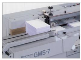
The automatic bottom-feed system allows for continuous top loading and production. (for 5 to 15 mm / 0.2" to 0.6" thickness book blocks)
