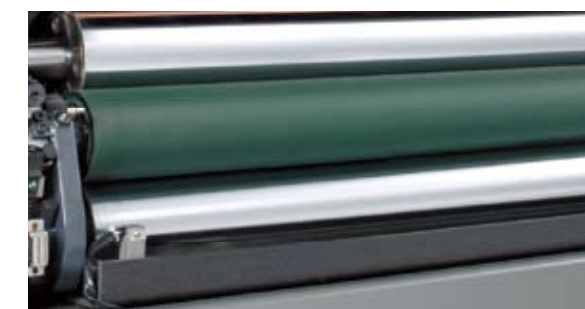
Komorimatic and ink/dampening roller configuration
