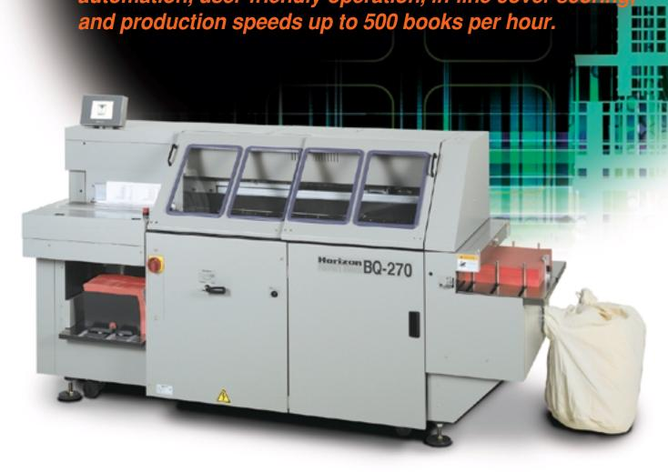
Even though the BQ-270 is a single clamp compact binder, it produces square accurate spines. The quality of bind on the BQ-270 is equal to that provided by more expensive multiple-clamp binding systems.
