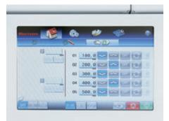
Newly equipped high resolution touchscreen provides intuitive operation. Changeovers including fold pattern, creasing number and up / down crease selection can be done easily at this screen. Up to 200 jobs can be stored in memory for easy recall.
