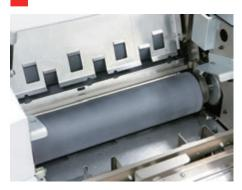
The large-diameter fold rollers are equipped for heavier stocks. Folding patterns include parallel fold, short fold, letter fold, double parallel fold, accordion fold, and open gate fold.
