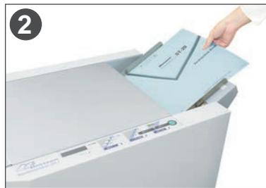
2 Insert prints, align the side guide, then press the start button. The booklets are produced immediately.
