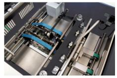
The servo-motor is employed for knife driving to provide high speed and sharp fore-edge trimming. The topbottom transport belt insures smooth booklet transportation and delivery. Trimmings are blown down into the external trim box by air so that no chips are left in the trimming area. Durable casting structure for quality trimming.
