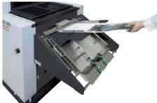
The IFU-200 allows hand feeding of previously collated sets, heavy cover material or difficult stocks in three modes.
