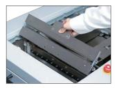
Perforation can be installed in the creasing section. A wide variety of creasing blades are available for different perforating patterns.
